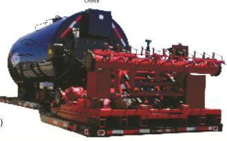
The RaynMaker's built in full-sweep agitator makes modifying sealcoat materials easy. Various latex products, SBS, SBR, tire rubber compounds and additional fine aggregates can be easily added, mixed and applied.
